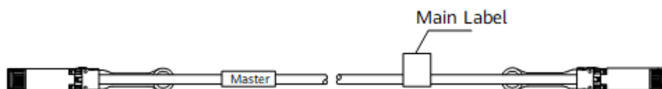
Figure 7-25 Dedicated stack cable structure
