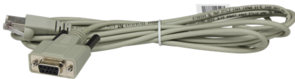
Figure 7-11 Appearance of a console cable
