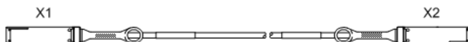
Figure 7-22 Structure of a QSFP+ to QSFP+ or QSFP28 to QSFP28 high-speed cable
